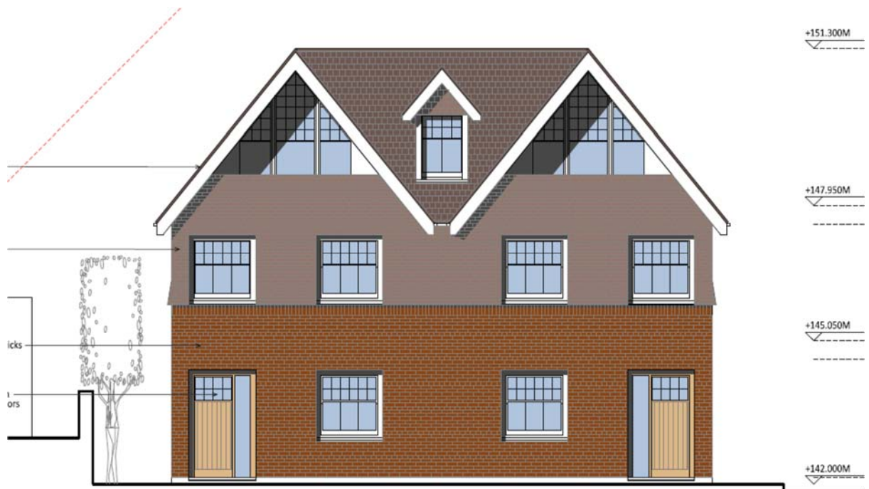
Fig 4.Semi-Detached Dwellings Front Elevation
